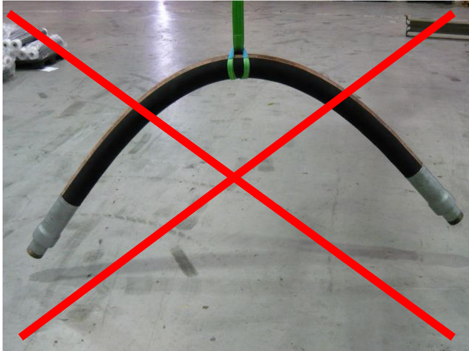
Figure 9: Incorrect moving and lifting of swaged hose
