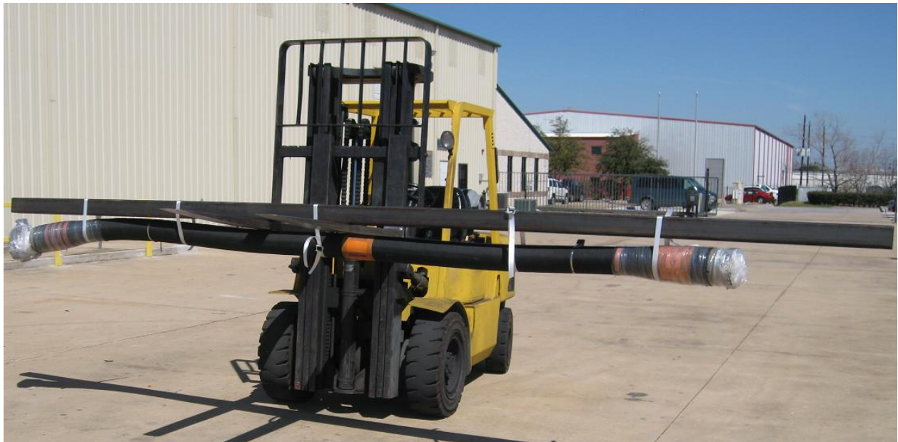
Figure 3: Using a lifting bar with straps and shackles to lift a hose.
