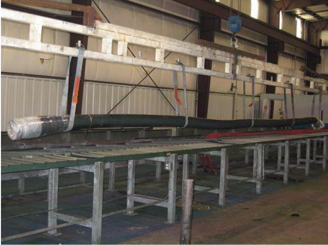
Figure 2: Using a lifting beam with straps to lift a hose.
