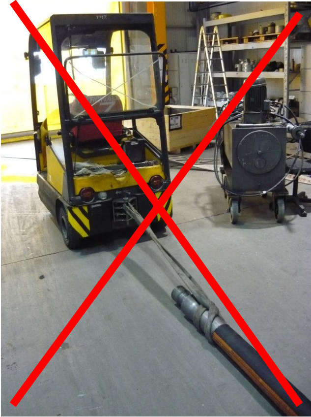
Figure 6: Inadmissible dangerous mode of transport by dragging hose across the ground
